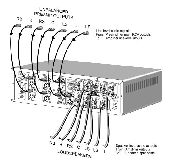
If your preamplifier has RCA outputs, it can be connected to the amplifier inputs as shown. The amplifier will boost the preamplifier's output, up to a level suitable for driving speakers.
